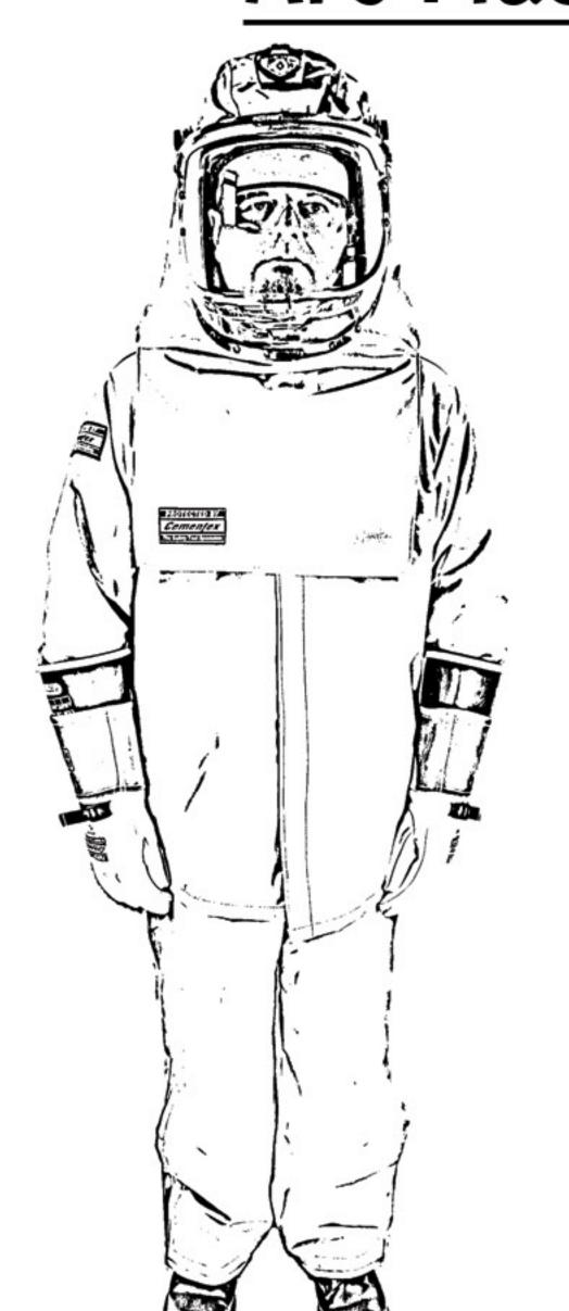
Arc-Rated Clothing selected so the system's Arc Rating meets the required Minimum Arc Rating of 40 cal/cm² (167.5J/cm²)
